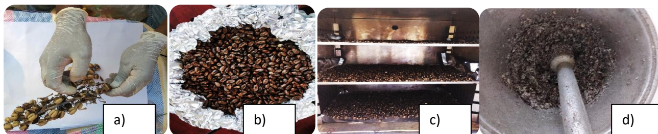
Fig.2. a) Dehusking;b) Drying with the sun;c) drying with the drying oven ;d) crushed Castor seeds
