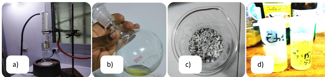
Fig.3 a) Assembly of the extractor soxhlet ; b) Mix extracted oil + hexane; c) Oil cakes; d) Castor oil extracted
