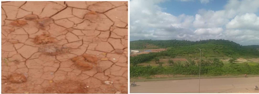
Figure 4: Shrinkage crack characteristic of silty soils (A), a panoramic view of relief of the study area (B)
