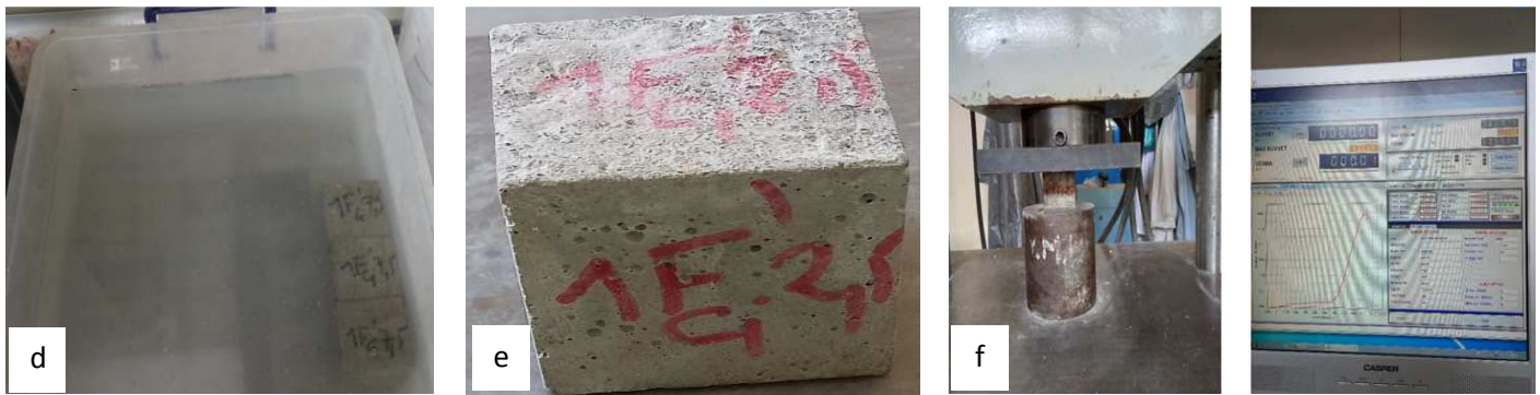
Figure 2: Rice husk a), unground rice husk ash b), ground rice husk ash c), mortar curing conditions d), unground rice husk ash specimen e), compression test equipment f).
