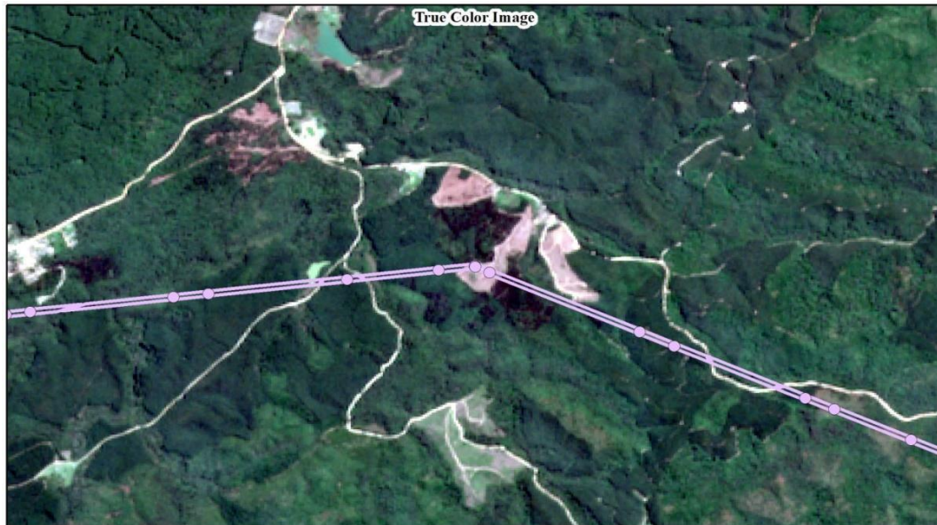
Figure 5: Towers and safety clearance of TL Novo Horizonte over the RGB composition of the multispectral image (Sentinel-2).
