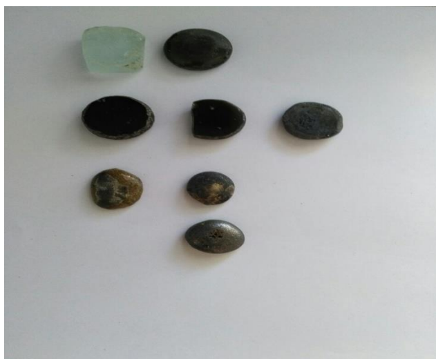
Fig.2: Samples of prepared glass and glass-ceramic
