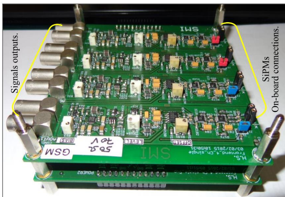
Fig. 4: A picture of the prototype detector system PCB circuit board, with built-in bias control, discriminator and signal offset level control. On board SiPMs current monitoring connections is visible.
