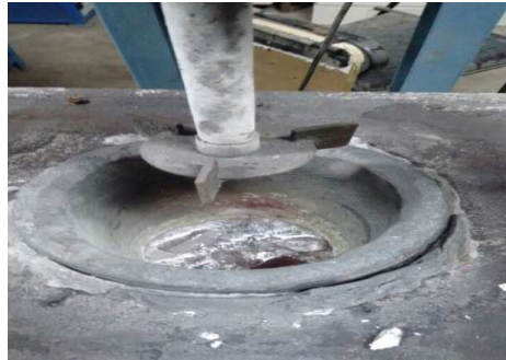
Fig. 6: Stir casting of aluminium alloy LM6 and preheated reinforcement.
