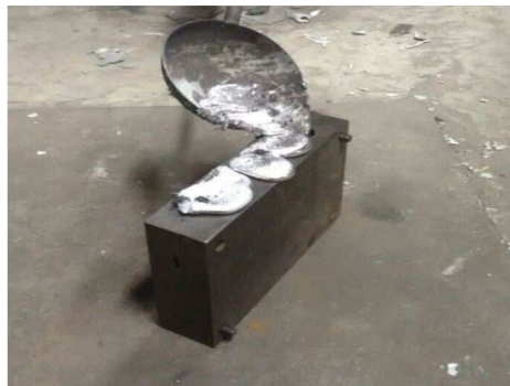
Fig. 6: Stir casting of aluminium alloy LM6 and preheated reinforcement.
