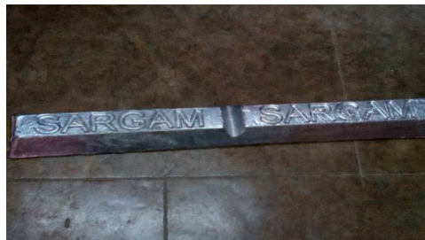
Fig. 3: Raw material of aluminium alloy LM6.
