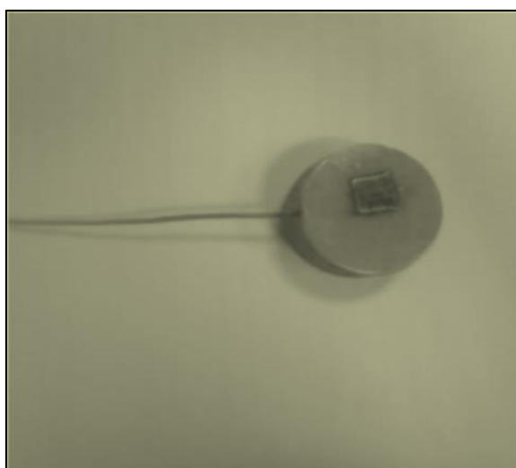
Fig. 1: Shows the photograph of the prepared mounted 316L SS samples.
