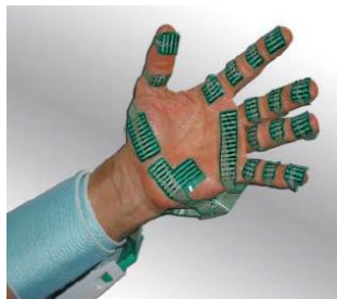
Fig. 2: Tactile Grip and Pressure Measurement (Grip System) by Tekscan.
