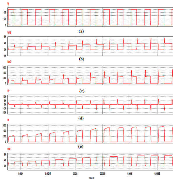
Fig. 5: Simulated switching waveforms of proposed converter under DCM.
