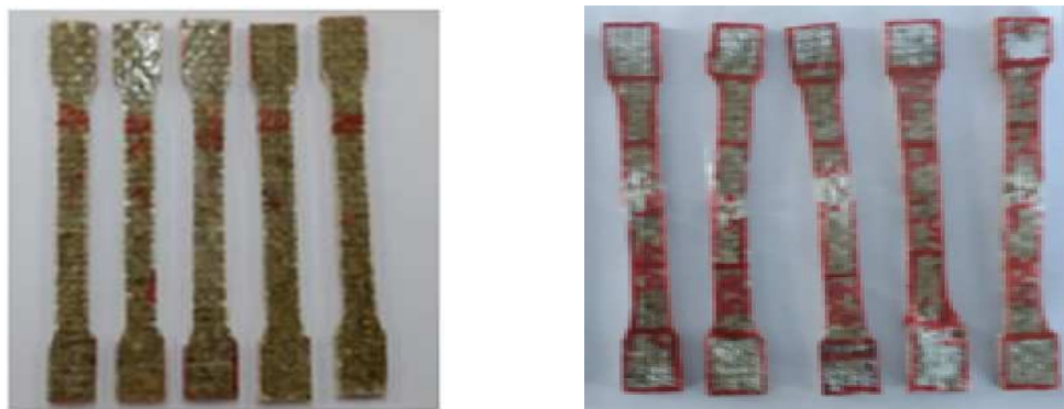
Fig. 2: View of tensile test specimen (a) before test (b) after test
