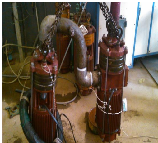
Fig. 5: Motor and subassemblies of submersible pump.
