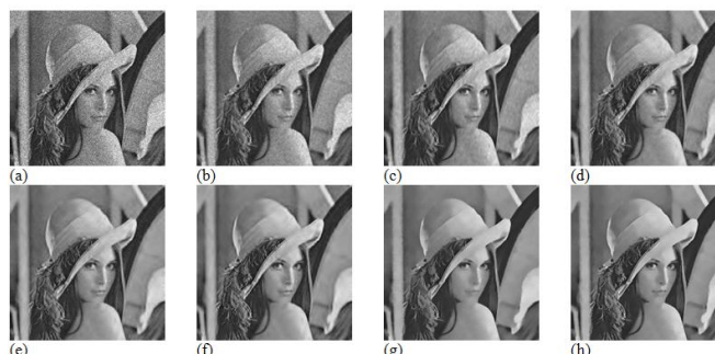
Fig. 5: Synthetic Image Denoising. (a) Noisy Image, (b) PPB, (c) NL – SAR, (d) Bilateral NLM, (e) Bayesian NLM, (f) Pretest NLM, (g) BM3D, (h) NL – CV.
