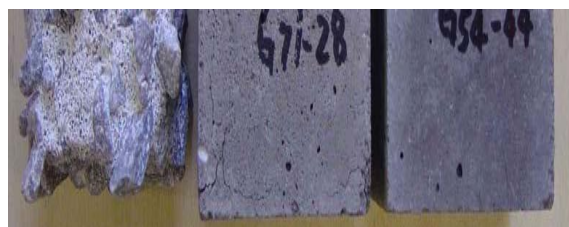
Fig. 2: Appearance of concrete specimens exposed in 10% sulphuric acid –Left Control Concrete for 28 days, right-Alkali activated concrete for 56 days (XJ Song)
