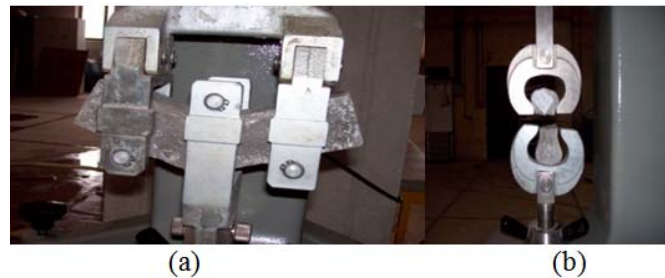
Fig. 4: Physical characteristics of mortars test: (a) flexural test (b) tensile test
