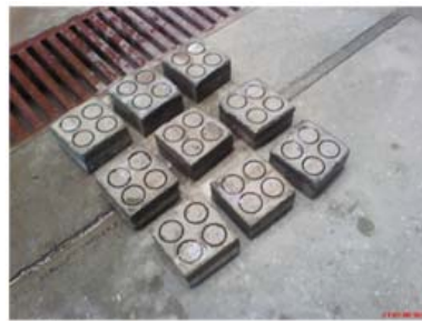
Fig 3: the specimens for testing by pull-off and friction transfer method
