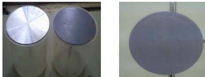
Fig. 2: PTFE : Disk Covered by PTFE sheet pasted on Aluminum Disk by pressing.
