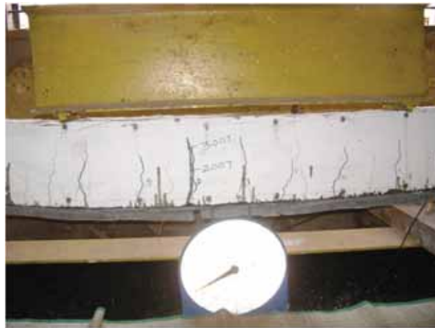
Fig. 10: Typical crack pattern of strengthened beam after failure
