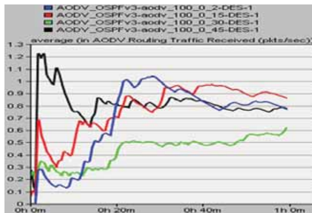
Fig. 4: Routing Traffic Received-Pause Time= 0 Second
