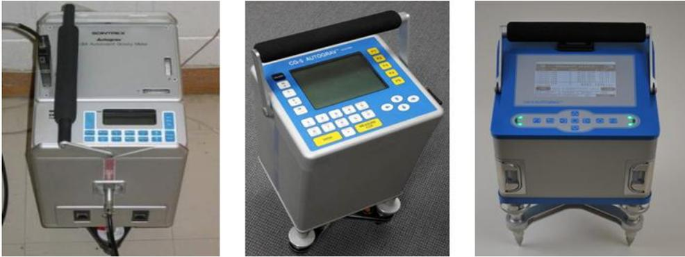
**Figure 1.** The three developed Scintrex Autograv gravimeters. From left to right: CG3/3M, CG-5, and CG-6.
