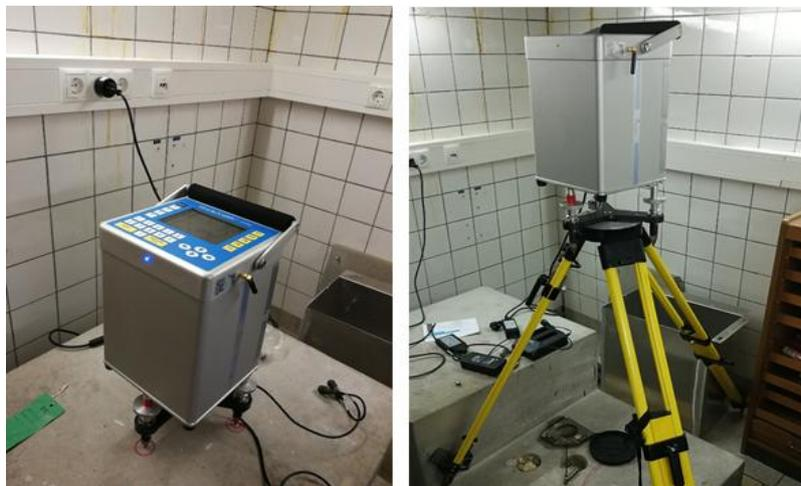
**Figure 2.** The Scintrex CG-5 Autograv of the UB-IGG gravity station installed on a pillar (left) and on a tripod (right).
