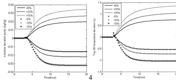
**Fig. 7:** Step test results for bottom composition (left) and Tray 68 temperature (right) by manipulating the *n*-butane feed composition at  $\pm 5\%$ ,  $\pm 10\%$  and  $\pm 15\%$  change from the nominal condition
