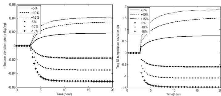
**Fig. 6:** Step test results for bottom product purity (left) and temperature Tray 68 (right) by manipulating the reboiler duty at  $\pm 5\%$ ,  $\pm 10\%$  and  $\pm 15\%$  change from the nominal condition
