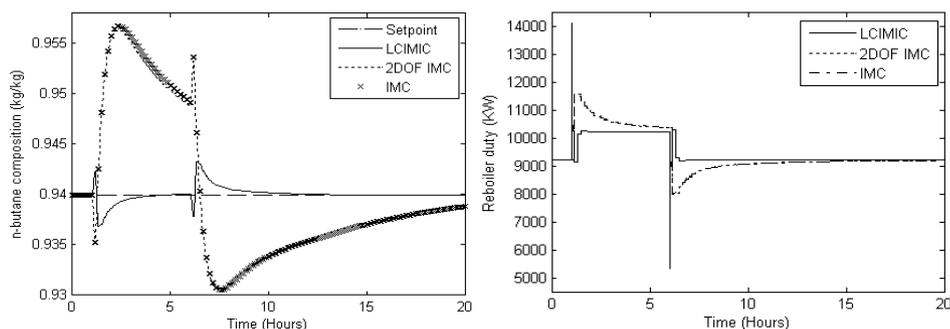
**Fig. 10:** Input disturbance rejection results for CIMIC, 2DOF IMC and IMC (left) Input disturbance rejection MV profile for CIMIC, 2DOF IMC and IMC (right)
