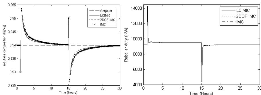
**Fig. 11:** Output Disturbance rejection results for CIMIC, 2DOF IMC and IMC (left) MV profile for CIMIC, 2DOF IMC and IMC output disturbance rejection test (right)
