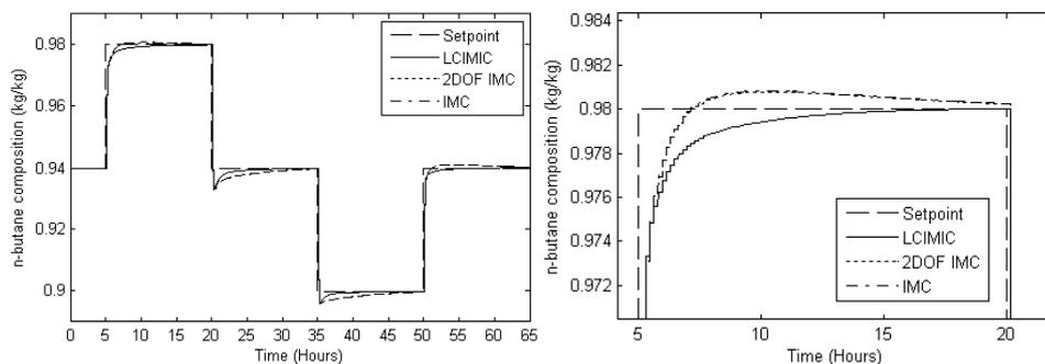
**Fig. 8:** Set point tracking response results for CIMIC, 2DOF IMC and IMC (left) Set point tracking result for a step up change at  $t=5$  hours (right)
