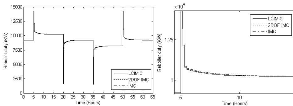
**Fig. 9:** Set point tracking MV profile results for CIMIC, 2DOF IMC and IMC (left) MV profile for step up at  $t=5$  hours (right)
