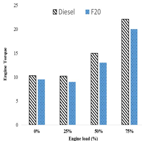
**Fig. 3:** Variation torque for Diesel and F20
