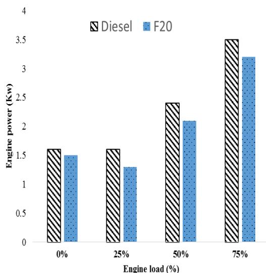
**Fig. 2:** Variation of power for Diesel and F20
