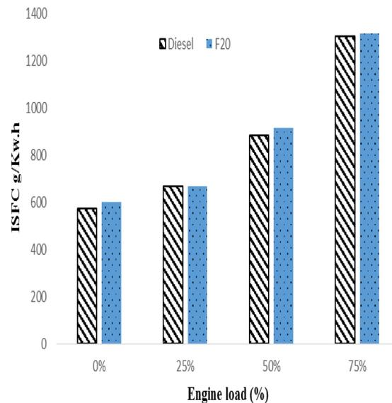
Fig. 5: Variation ISFC of diesel and F20
