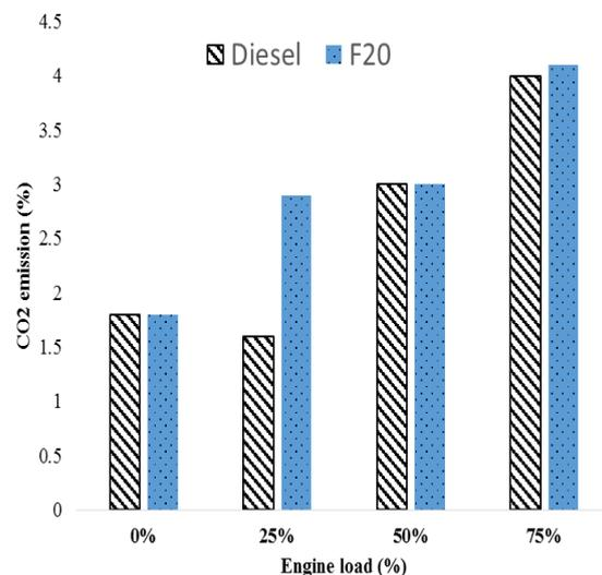
Fig. 8: Variation CO<sub>2</sub> emission of diesel and F20
