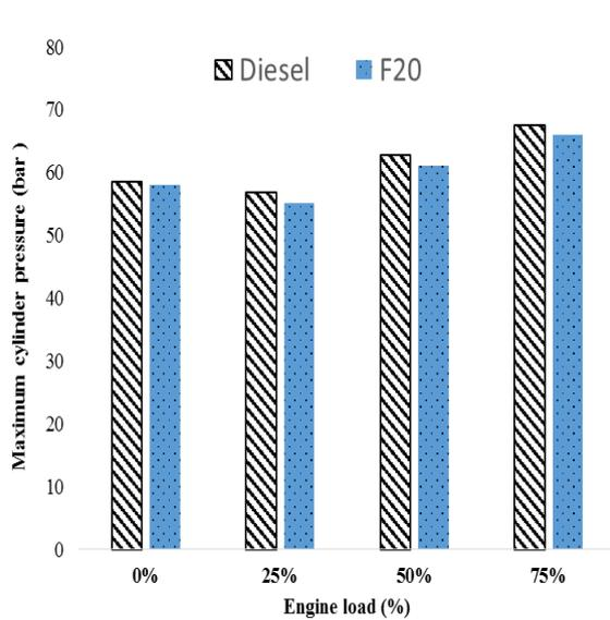
Fig. 4: Variation MCP of diesel and F20
