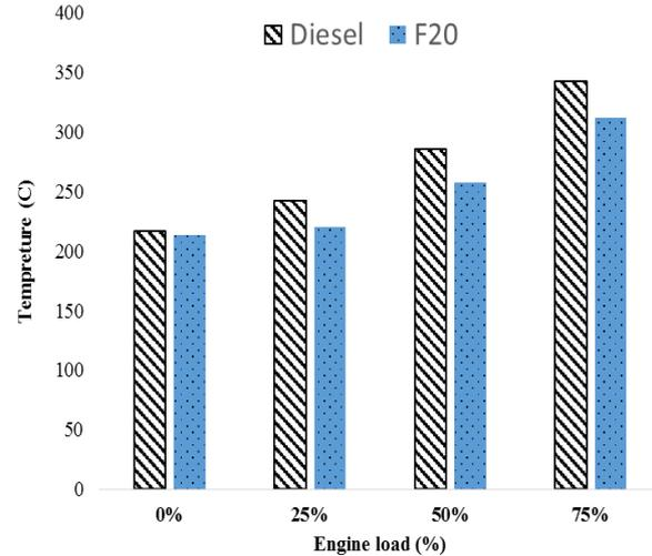
Fig. 7: Variation exhaust temperature of diesel and F20
