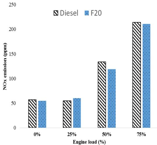
Fig. 6: Variation NO<sub>x</sub> emission of diesel and F20
