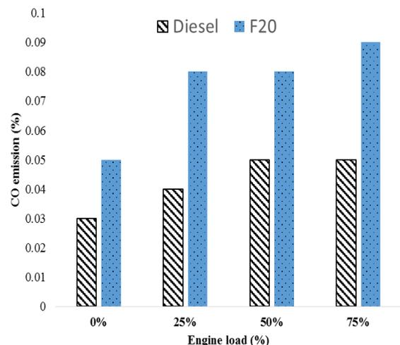
Fig. 9: Variation CO emission of diesel and F20
