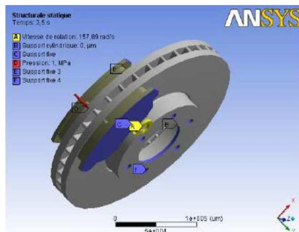
Fig. 5: Boundary conditions and loading imposed on the disc pads (Ali Belhocine and M. Bouchetra 2014).
