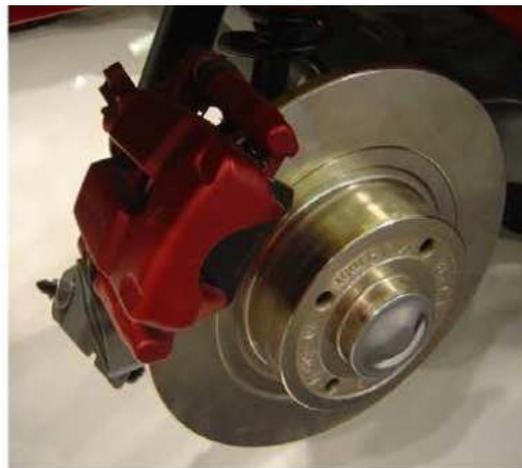
**Fig. 2:** Solid Disc Brake (Talati and Faramarz, 2009)
