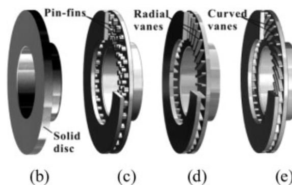
**Fig. 3:** Schematic illustration of car disc brake system (b) solid disc brake type (c) - (e) ventilated brake discs type pin-fins, radial vanes and curved vanes (T.C. Charterley *et al.*, 1999)
