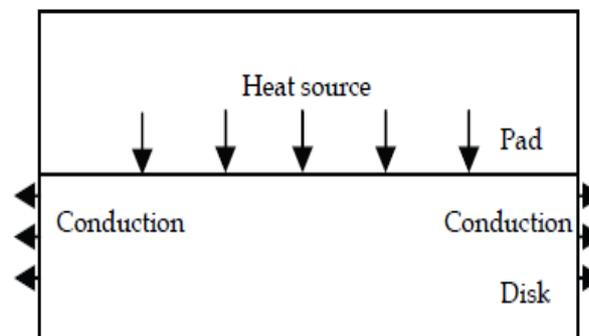
**Fig. 1:** Heat transfer boundary conditions (M. Eltoukhy, 2008).
