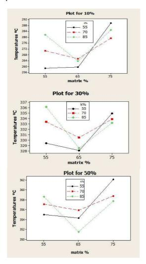
Fig. 3: TGA resultsTGA temperatures results for (10%, 30% and 50%) of degradations
