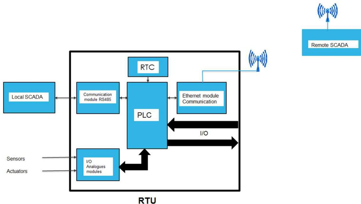
**Fig. 1:** The block diagram of the proposed R.T.U
