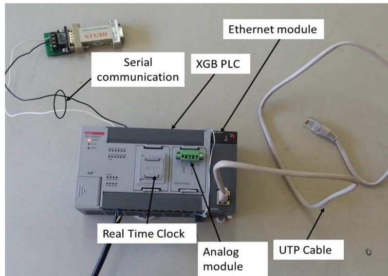
**Fig. 5:** the designed and successfully Implemented RTU
