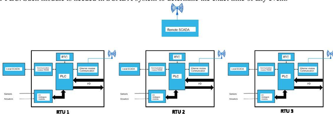
**Fig. 2:** Remote SCADA communicating with multiple RTUs in different Locations via Ethernet Modules
