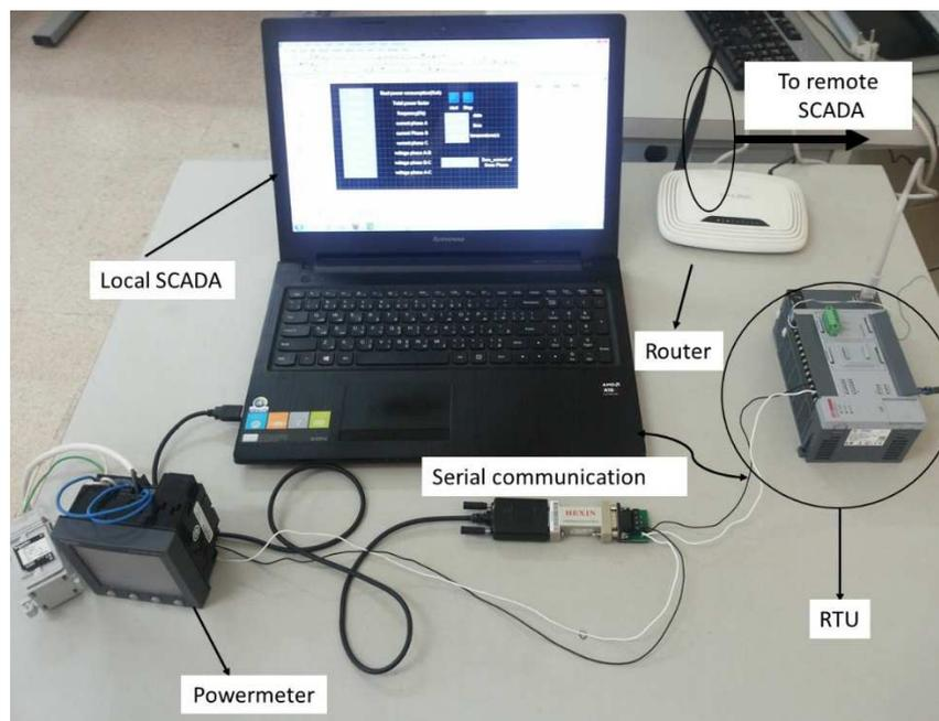
**Fig. 6:** Local SCADA Communicating with the RTU and the Power Meter
