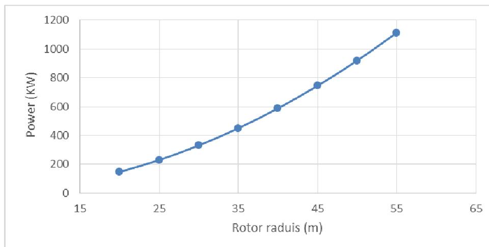
**Fig. 6:** relation between output power and rotor radius
