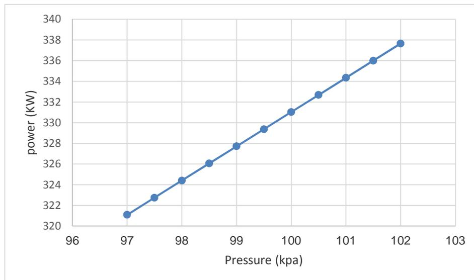
**Fig. 8:** relation between pressure and power in Jordan conditions
