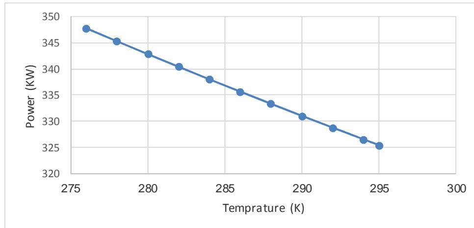
**Fig. 7:** relation between power an temperature in Jordan conditions
