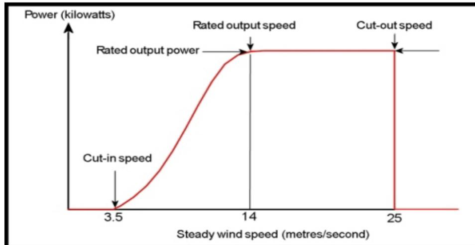
Fig. 2: Typical wind turbine power output with steady wind speed (<http://www.wind-power-program.com/popups/powercurve.htm>)
