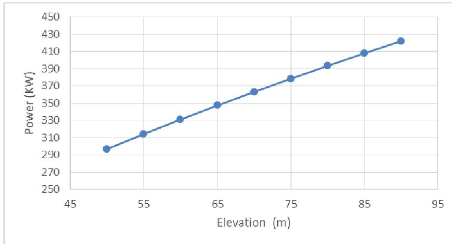
**Fig. 5:** output power Vs. turbine elevation
