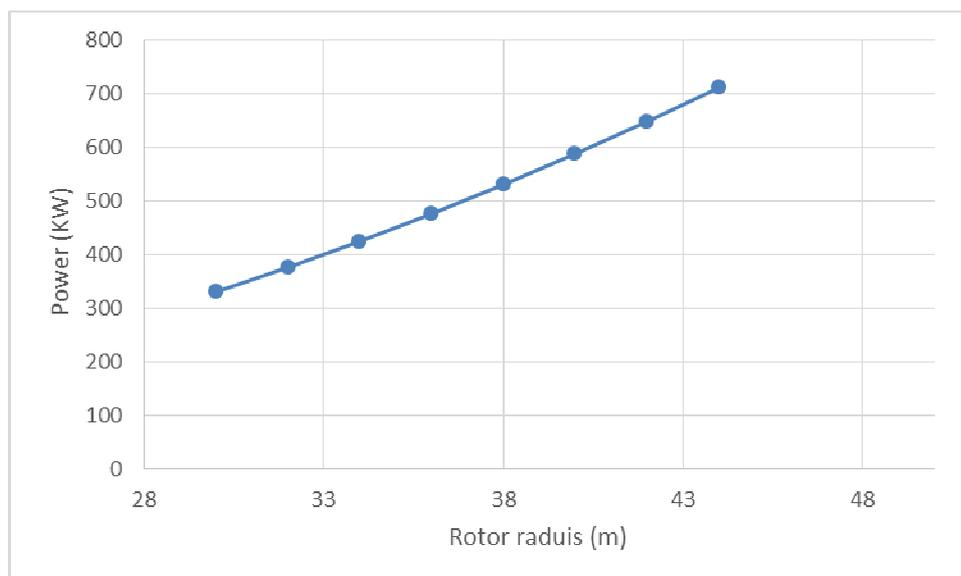
**Fig. 10:** relation between power and rotor radius in Jordan conditions
