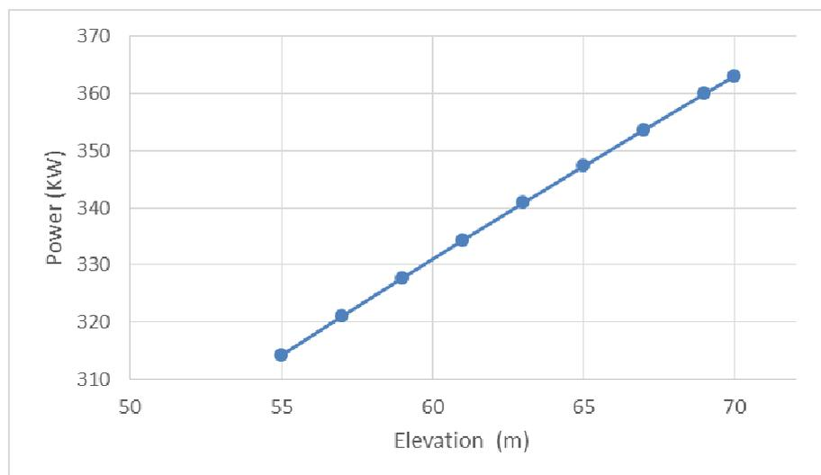
**Fig. 9:** relation between power and turbine elevation in Jordan conditions
