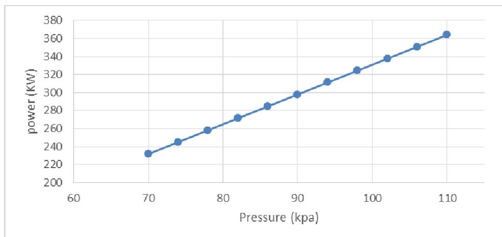
**Fig. 4:** pressure effect on out power
