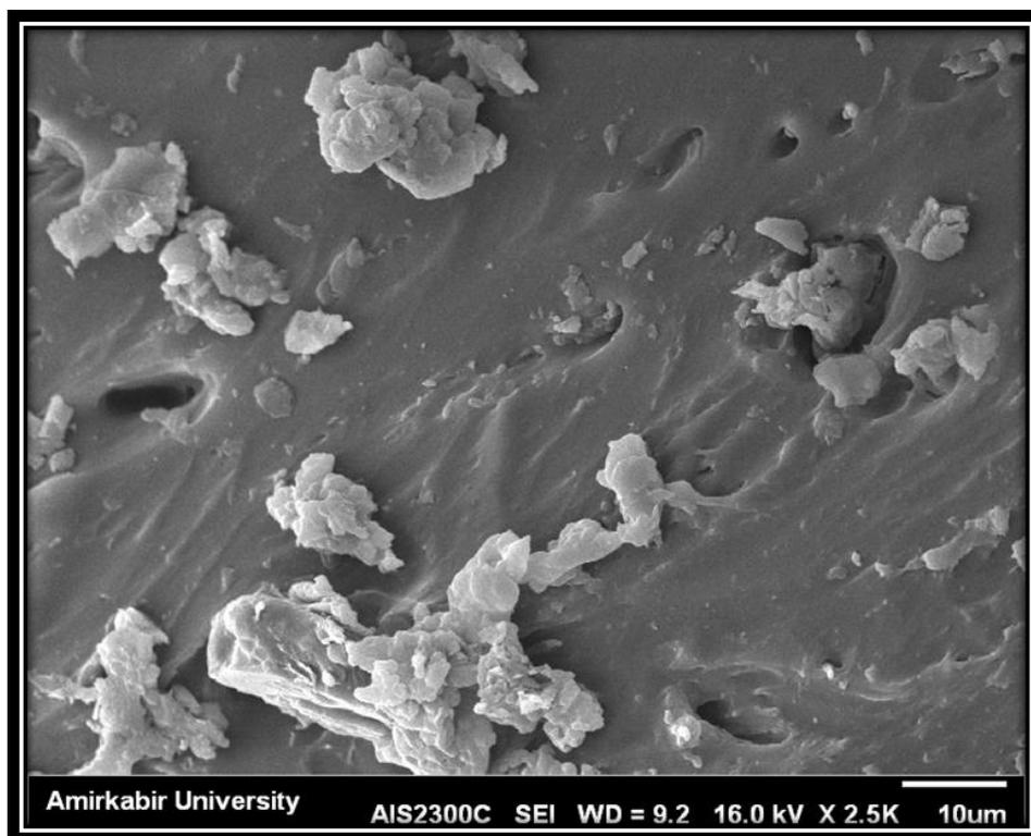
**Fig. 4-2:** SEM image of PVC composite containing ATH nanoparticles.
