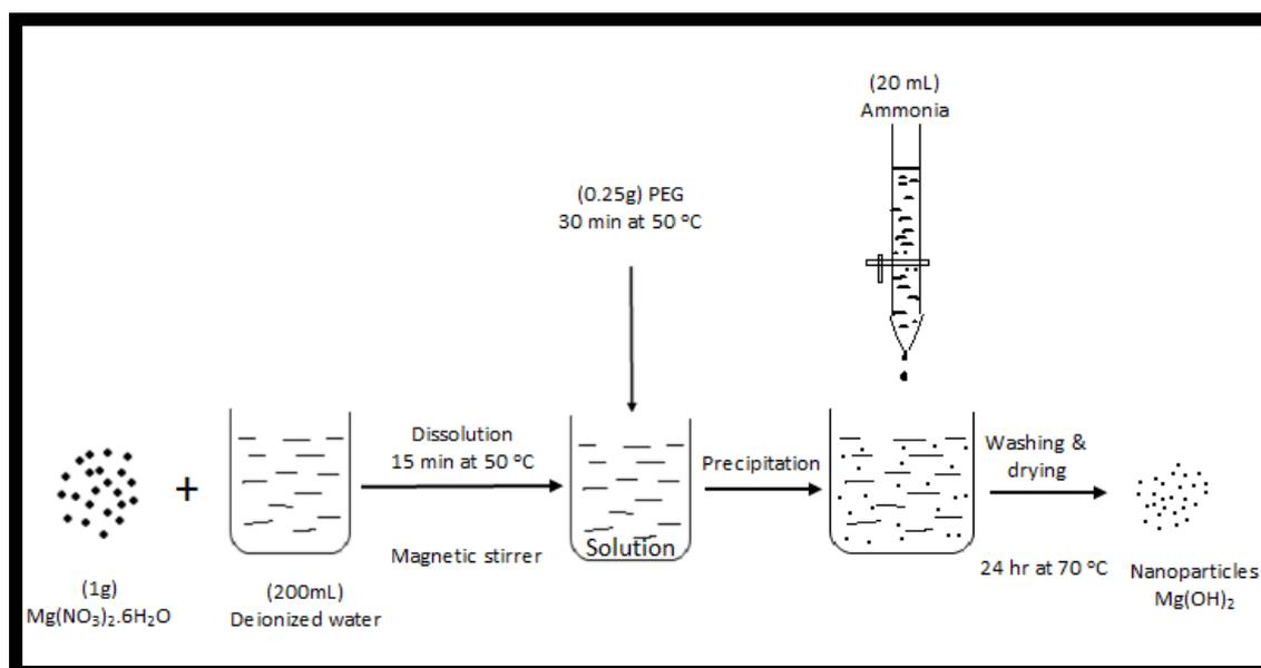
Fig. 2-1: Schematic diagram of  $Mg(OH)_2$  nanostructures Preparation.
