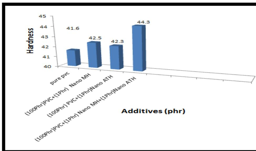
**Fig. 4-4:** Hardness for PVC nanocomposite that contain (MH),(ATH) and (MH+ATH).
