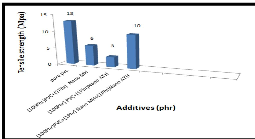
**Fig. 4-3:** Tensile strength for PVC nanocomposite that contain (MH),(ATH) and (MH+ATH).
