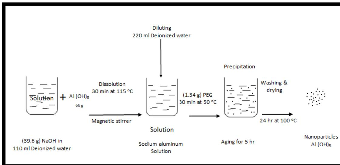
**Fig. 2-2:** Sketch of  $\text{Al}(\text{OH})_3$  nanostructures Preparation.
