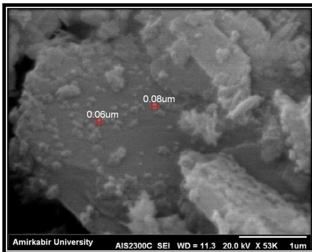
Fig. 2-6: Particle size of aluminum tri-hydroxide nanoparticle.
