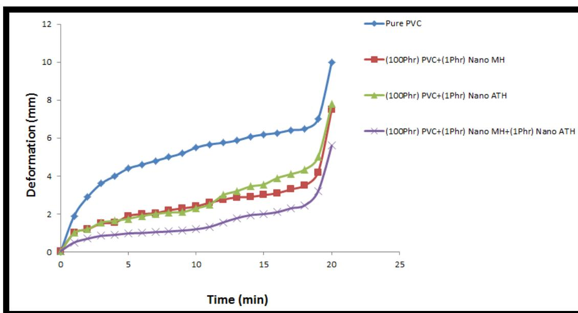
**Fig. 4-5:** creep of PVC nanocomposite that contain (MH),(ATH) and (MH+ATH) nanoparticles.
