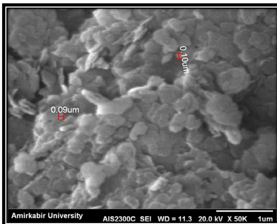
**Fig. 2-5:** Particle size of magnesium hydroxide nanoparticle.
