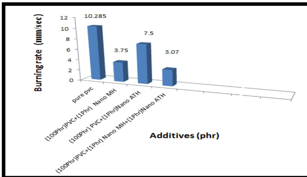
**Fig. 3.1:** burning rate of PVC nanocomposite, that contain(MH),(ATH)and (MH+ATH).
