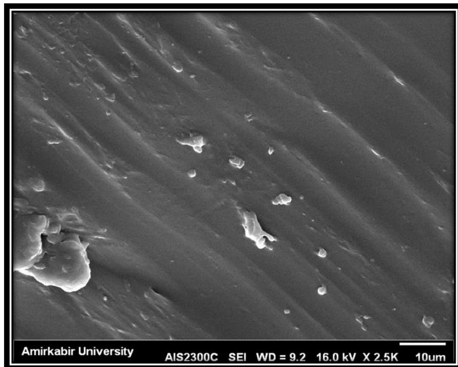
**Fig. 4-1:** SEM image of PVC composite containing MH nanoparticles.
