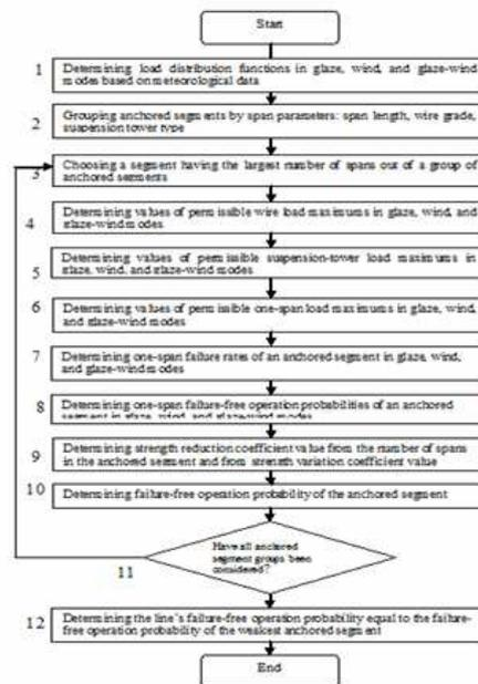
Fig. 1: Algorithm for reliability assessment of the mechanical OL section.
