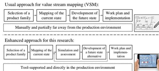
**Fig. 1:** Comparison of the work flows of VSM following the usual analytical approach and mobile value stream simulation.
