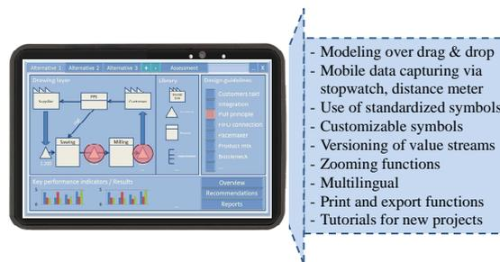
**Fig. 2:** Sketch of a possible user interface of a mobile value stream simulation tool and selected expert requirements.**Potentials Due To Smart Factory:**
