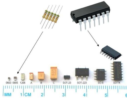
Fig. 6: Re-sizing of components.
