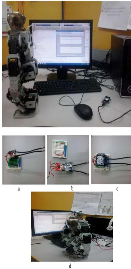
**Fig. 3:** a. Voltage and Current sensor, b. Voltage & current sensor with xbee, c. The transmitting remote circuit .d. the response of the robot
