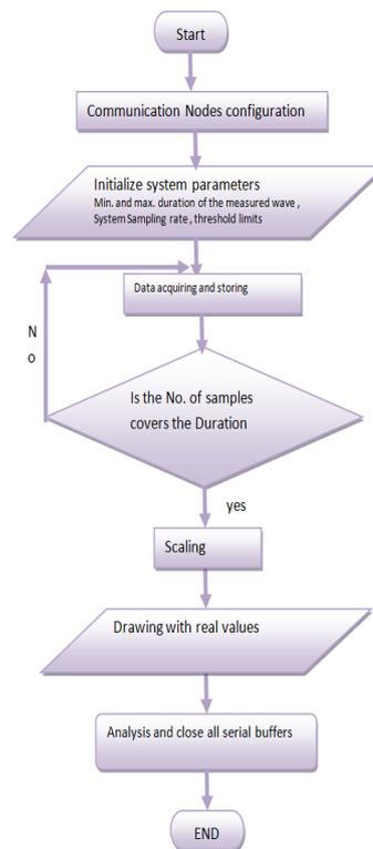
**Fig. 2:** Flow chart for the wireless communication between xbee and the robot.
