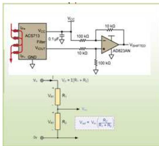
**Fig. 4:** Energy sensors signal conditioning.
