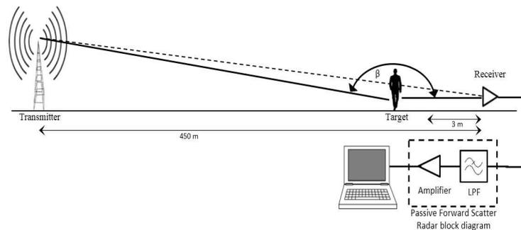
**Fig. 1:** Architecture of passive forward scattering radar system.
