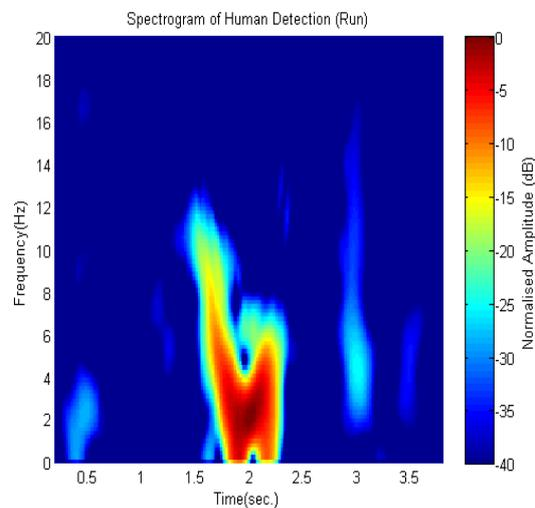
**Fig. 9:** Spectrogram of human detection while running.
