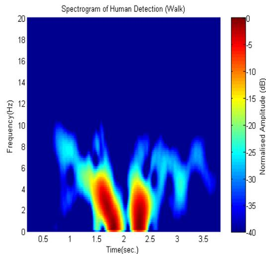
**Fig. 8:** Spectrogram of human detection while walking.
