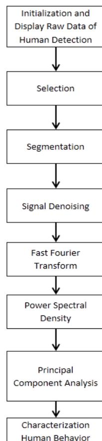
**Fig. 3:** Signal pre-processing block diagram of characterization human behavior in passive forward scattering radar system.
