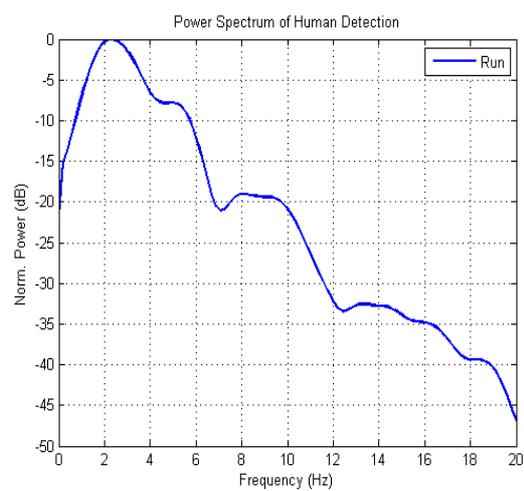
**Fig. 7:** Power spectrum density of human detection while running.
