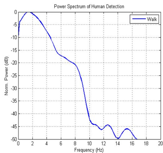
**Fig. 6:** Power spectrum density of human detection while walking.
