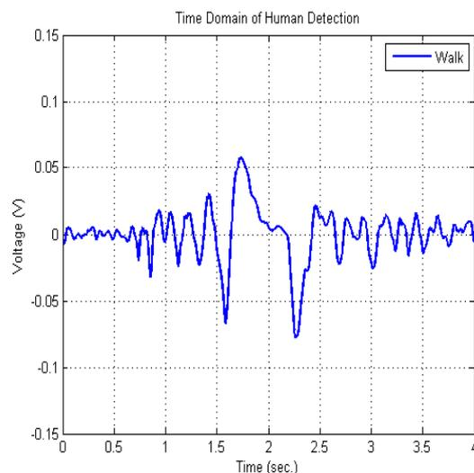
**Fig. 4:** Time domain of human detection while walking.
