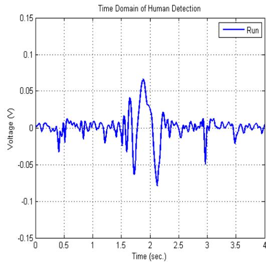
**Fig. 5:** Time domain of human detection while running.
