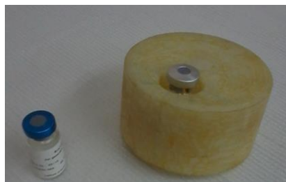
Fig. 3: Neck phantom and ^{131}\text{I} for measurement of efficiency detection.
