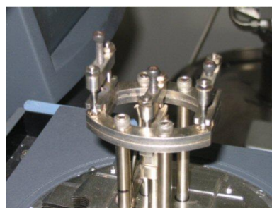
Fig. 3: The single cantilever mode for DMTA test.
