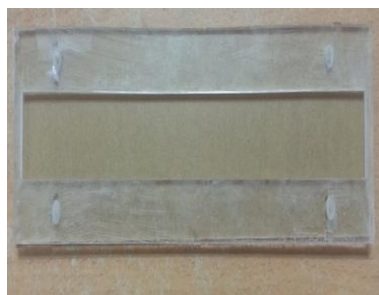
Fig. 1: Perspex mould used in manufacturing the epoxy resin.
