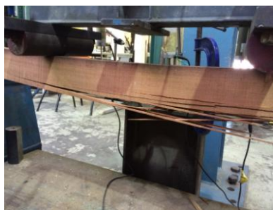
Fig. 8: Mode of failure on bending.
