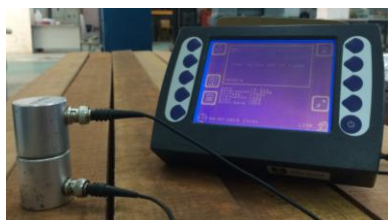
Fig. 4: Test equipment of UPV-E49 for NDT.
