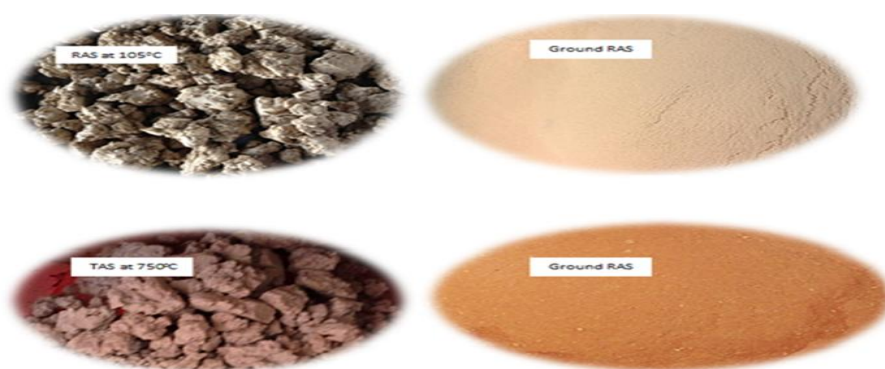
Fig. 3: Picture showing the alum sludge with treatment
