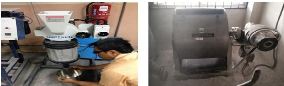
Fig. 2: Picture showing the dried AS and TAS was grounded using Cross Beater (Rotor Mill SK 100) and a Los Angeles abrasion test machine (LAAT) to get the necessary fineness.
