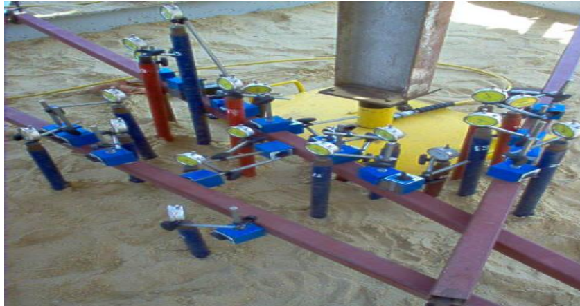
Fig. 3: Settlement readings using dial gauges.
