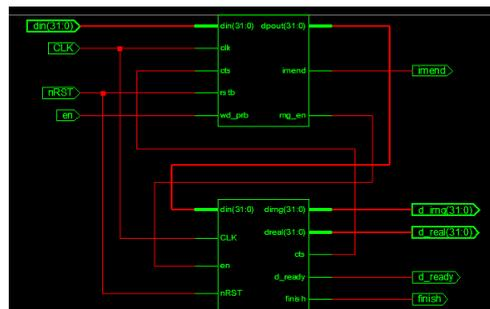
**Fig. 7:** RTL schematic of Gabor Filter with Real and Imaginary Kernel.
