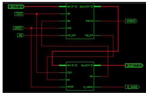
**Fig. 6:** RTL schematic of Gabor Filter with Real Kernel.
