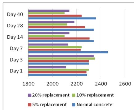
Fig. 2: The average total density for the prism test.
