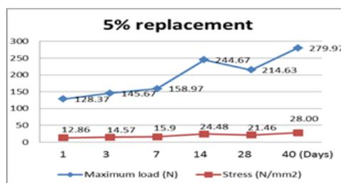
Fig. 4: 5% of cement replacement.
