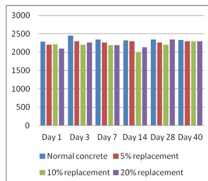
**Fig. 1:** The average total density for the cube test.
