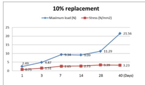
Fig. 9: 10% of cement replacement.
