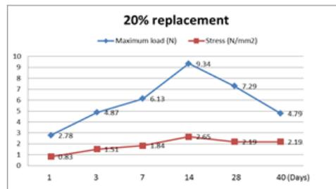
Fig. 10: 20% of cement replacement.
