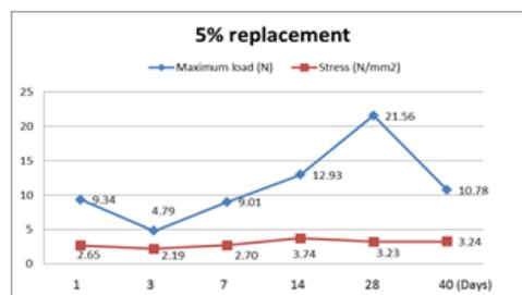
Fig. 8: 5% of cement replacement.
