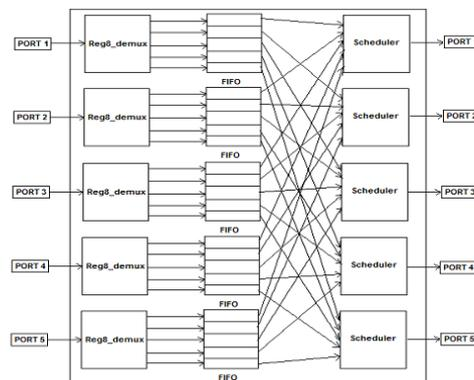
**Fig. 2:** shows the internal architecture of the designed router.
