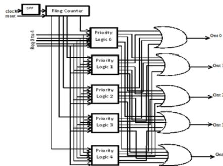
Fig. 4: Internal structure of arbiter .
