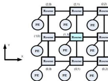
**Fig. 1:** Basic Networks on Chip architecture with mesh topology.
