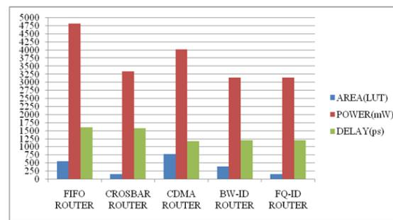
**Fig. 7:** Graphical Comparison on optimizing parameter (Area, power and Latency).
