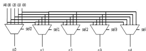
**Fig. 3:** Internal structure of crossbar.
