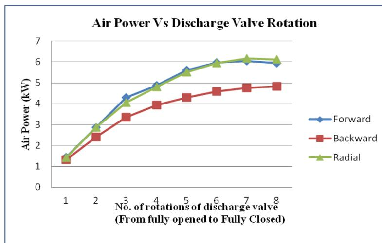
**Fig. 4:** Air Power Vs Discharge Valve Rotation of all blades.
