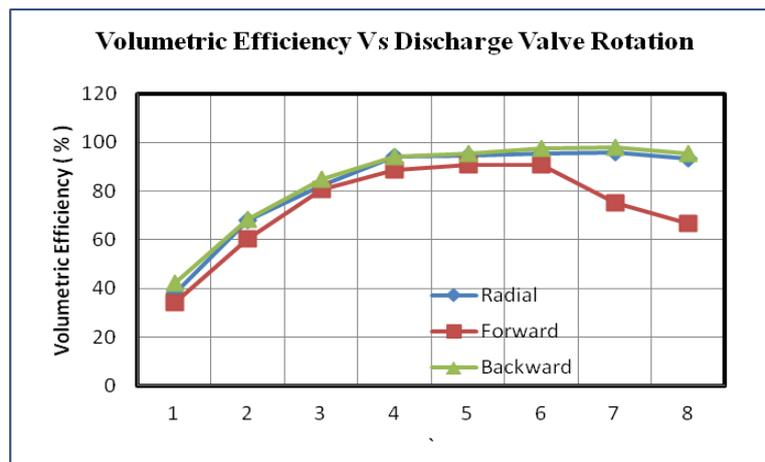
**Fig. 3:** Volumetric Efficiency Vs Discharge Valve Rotation of all blades.
