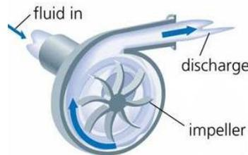
**Fig. 2:** Direction of air flow in blower.
