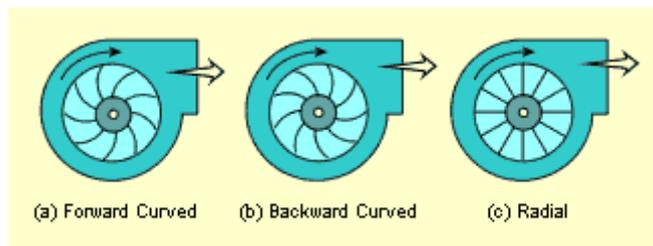
**Fig. 1:** Impeller blades of a blower.
