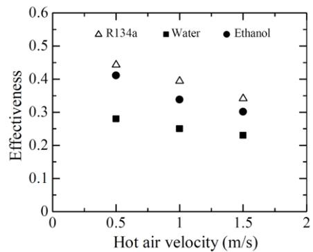
Fig. 6: Effect of hot gas velocity on effectiveness of CLOHP/CV heat exchanger.
