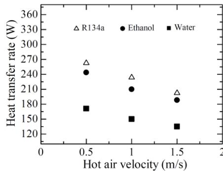
Fig. 5: Effect of hot gas velocity on heat transfer rate of CLOHP/CV heat exchanger.
