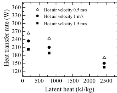
**Fig.7:** Effect of working fluid on heat transfer rate of CLOHP/CV heat exchanger.
