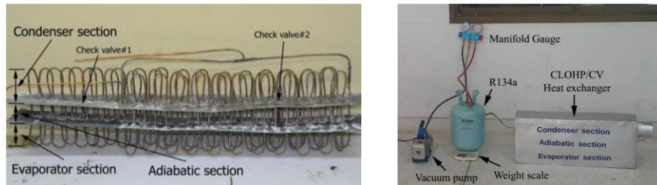
**Fig. 2:** The CLOHP/CV heat exchanger and working fluid charging.
