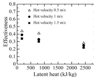
**Fig. 8:** Effect of working fluid on effectiveness of CLOHP/CV heat exchanger.
