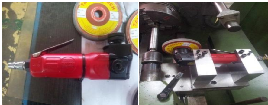
Fig. 3: Pneumatic hand grinder fitted on the bracket on lathe machine.
