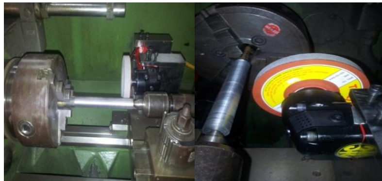
Fig. 5: Experimental set-up for grinding process of portable grinder.
