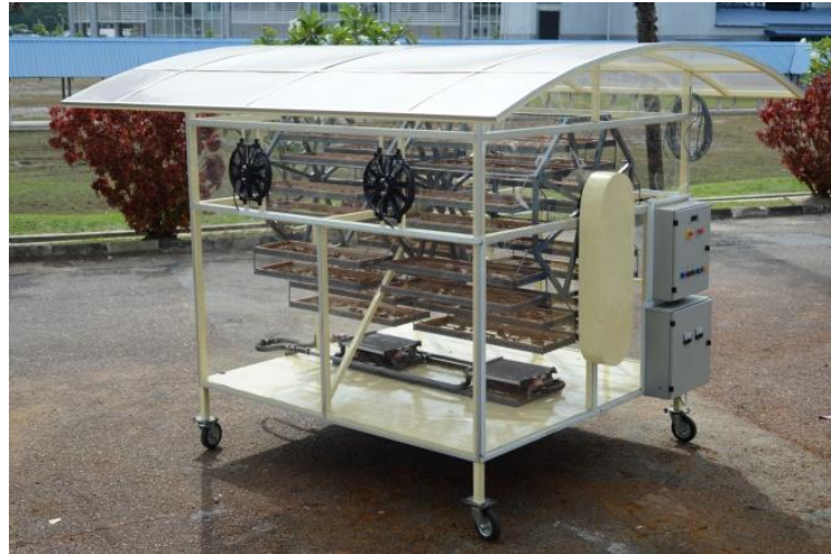
Fig. 1: An automated hybrid fish cracker dryer under running test
