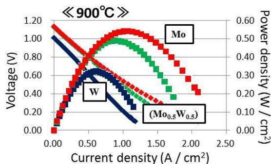
**Fig. 3:** Power generation at high temperature  $\text{Sr}_2\text{FeMoO}_{6-\delta}$  showed higher power density
