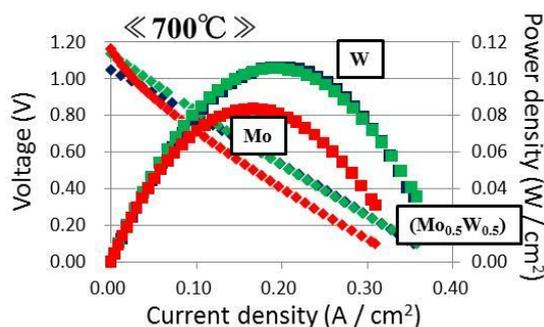
**Fig. 4:** Power generation at high temperature.  $\text{Sr}_2\text{FeWO}_{6-\delta}$  showed higher power density
