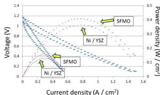
**Fig. 5:** Current-voltage and power density curves at  $700^\circ\text{C}$  and  $800^\circ\text{C}$  by comparison SFMO and Ni/YSZ
