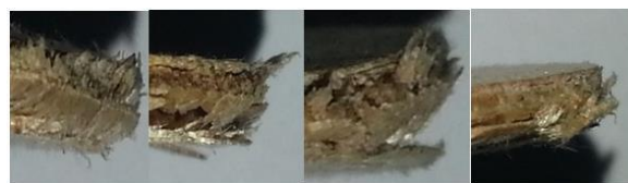
Fig. 3: Condition of cut edge at the bottom layer.
