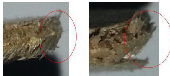
Fig. 2: Smallest cutting clearance (left) & biggest cutting clearance (right).
