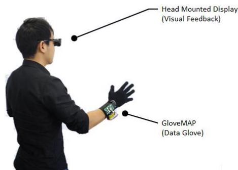
**Fig. 7:** Propose system of hand rehabilitation
