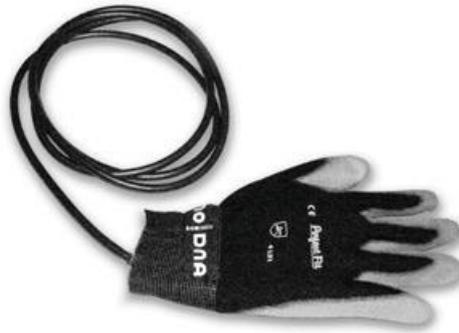
**Fig. 1:** X-IST CyberGlove made by Immersion Corp.
