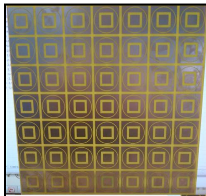
Fig. 3: Measurements setup showing the design double slot FSS structure positioned between two horn antenna
