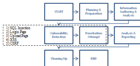
Fig. 6: UiTM Pahang web application penetration testing process.
