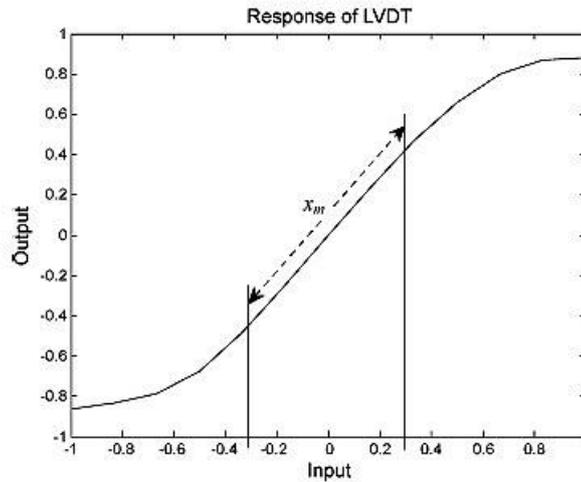
**Fig. 2:** Range of linear region of LVDT
