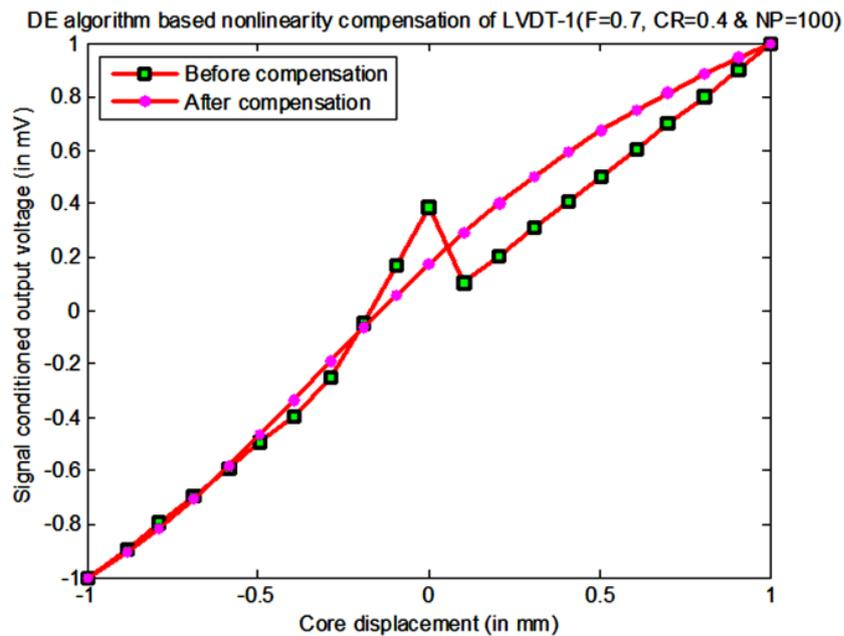
**Fig. 8:** DE algorithm based nonlinearity compensation of LVDT-1 (F=0.7, CR=0.4 & NP=100)
