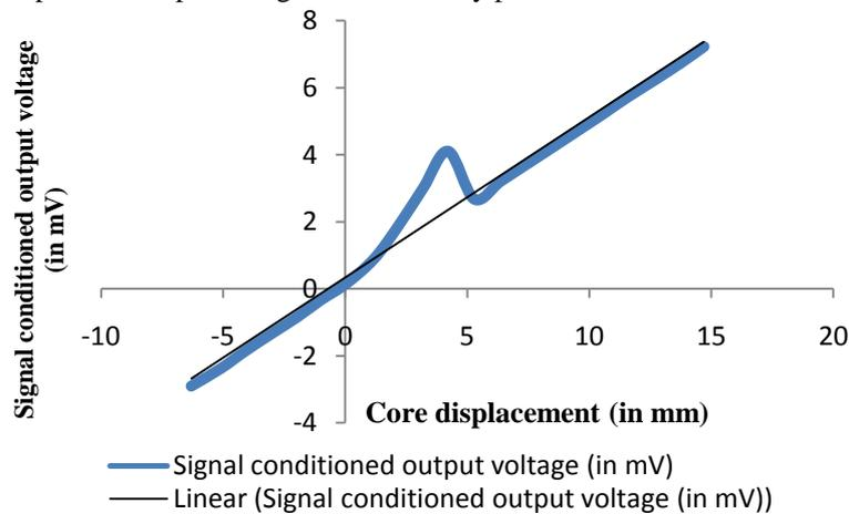
**Fig. 4:** Input-Output Response of LVDT-1
