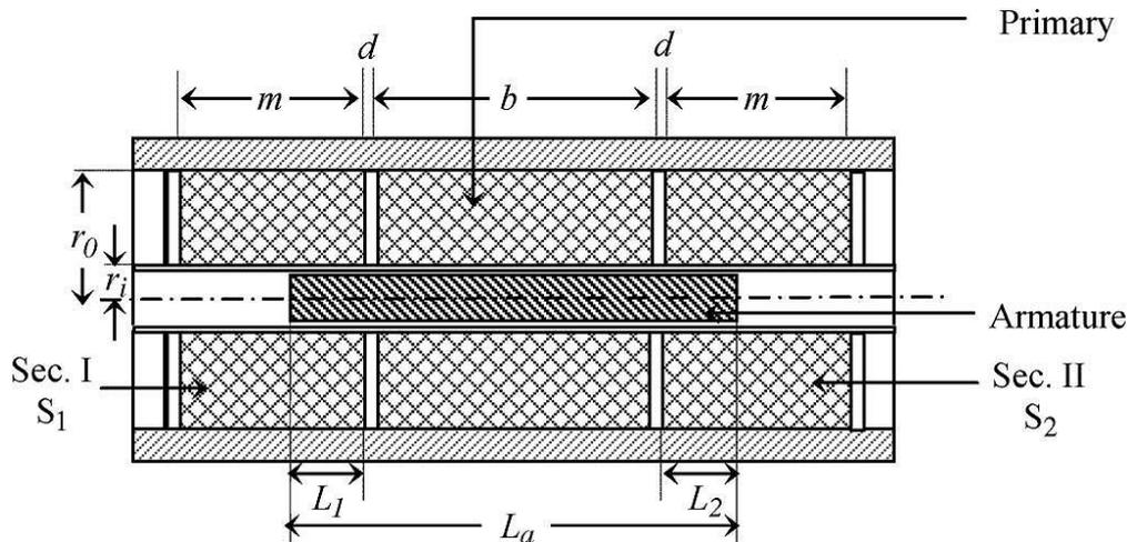
**Fig. 1:** Cross-sectional view of LVDT.
