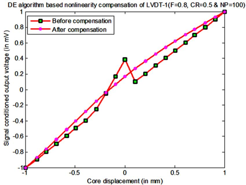
**Fig. 7:** DE algorithm based nonlinearity compensation of LVDT-1 (F=0.8, CR=0.5 & NP=100)
