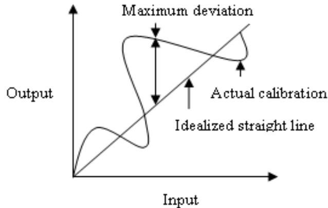
**Fig. 3:** Actual calibration curve
