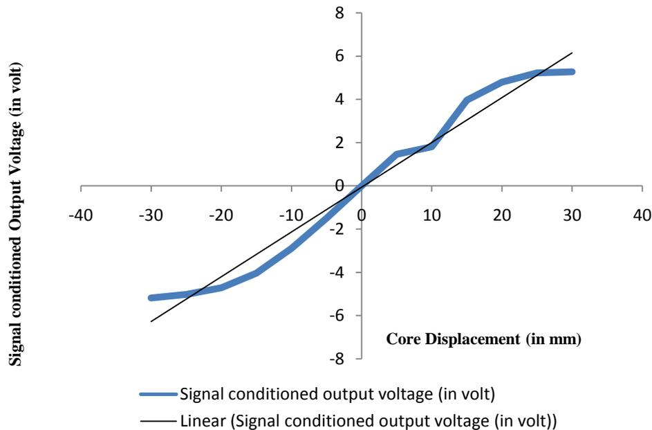
**Fig. 5:** Input-Output Response of LVDT-2
