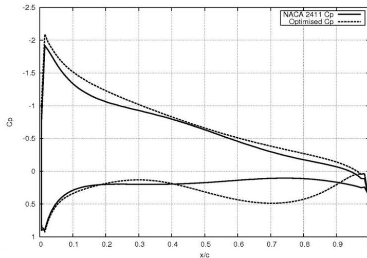
**Fig. 5:** Comparison of pressure distribution over the surface of original NACA 2411 airfoil and Optimized Airfoil.
