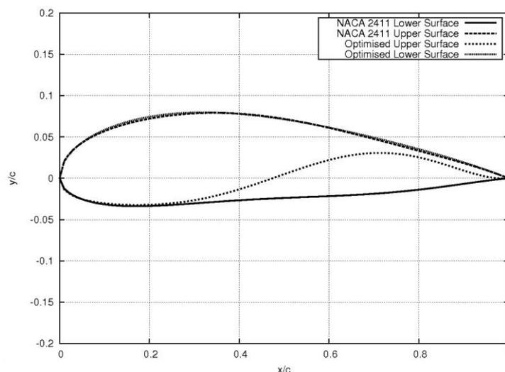
**Fig.4:** Original NACA 2411 airfoil Vs Optimized Airfoil.
