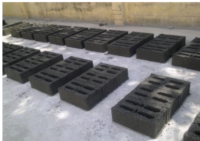
Fig. 5: Hollow Concrete Blocks Cast and Tested.
